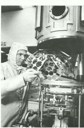
JEFF TINGLEY (2141) prepares planetary wafer fixture for deposition of aluminum on the wafers by evaporation inside a vacuum system.
